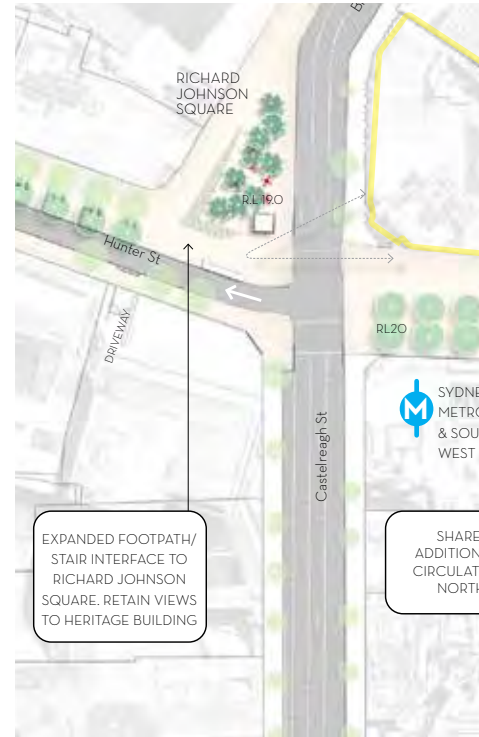
Concept plan showing enlarged Richard Johnson Square (Gallagher Studio Hunter Street Precinct Public Domain Strategy 2023)
